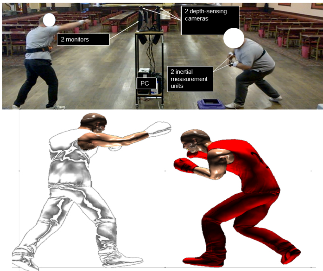
Figure 1. The exergaming system comprising hardware and software with real-time avatar mapping.
