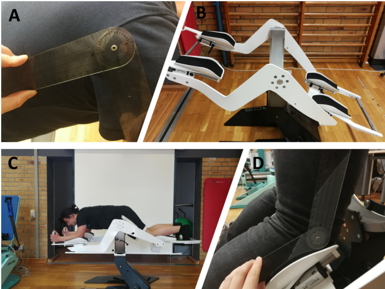
Figure 1. (A) Torso-arm angle measurement using protractor, (B) Icaros device, (C) participant being familiarized with the device, (D) upper-to-lower limb angle measurement using protractor.
