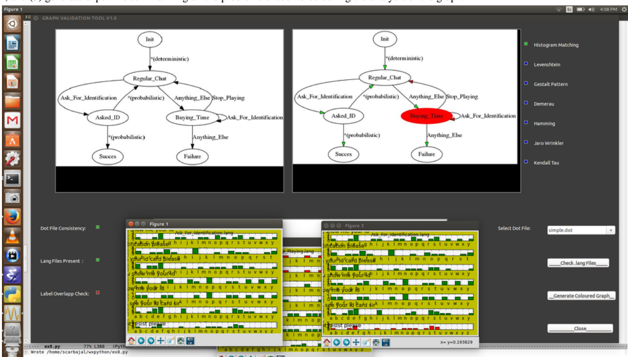
Figure 9. The main window of the graph validation tool. From this window, the user can (1) choose a Graphviz (.dot file) example to be analyzed, (2) obtain a graphic representation of the training exercise that it encodes, (3) select one of the available string metrics, (4) view letter histograms for each label, and (5) generate a .pdf file summarizing all the problems encountered during the analysis of the graph.
