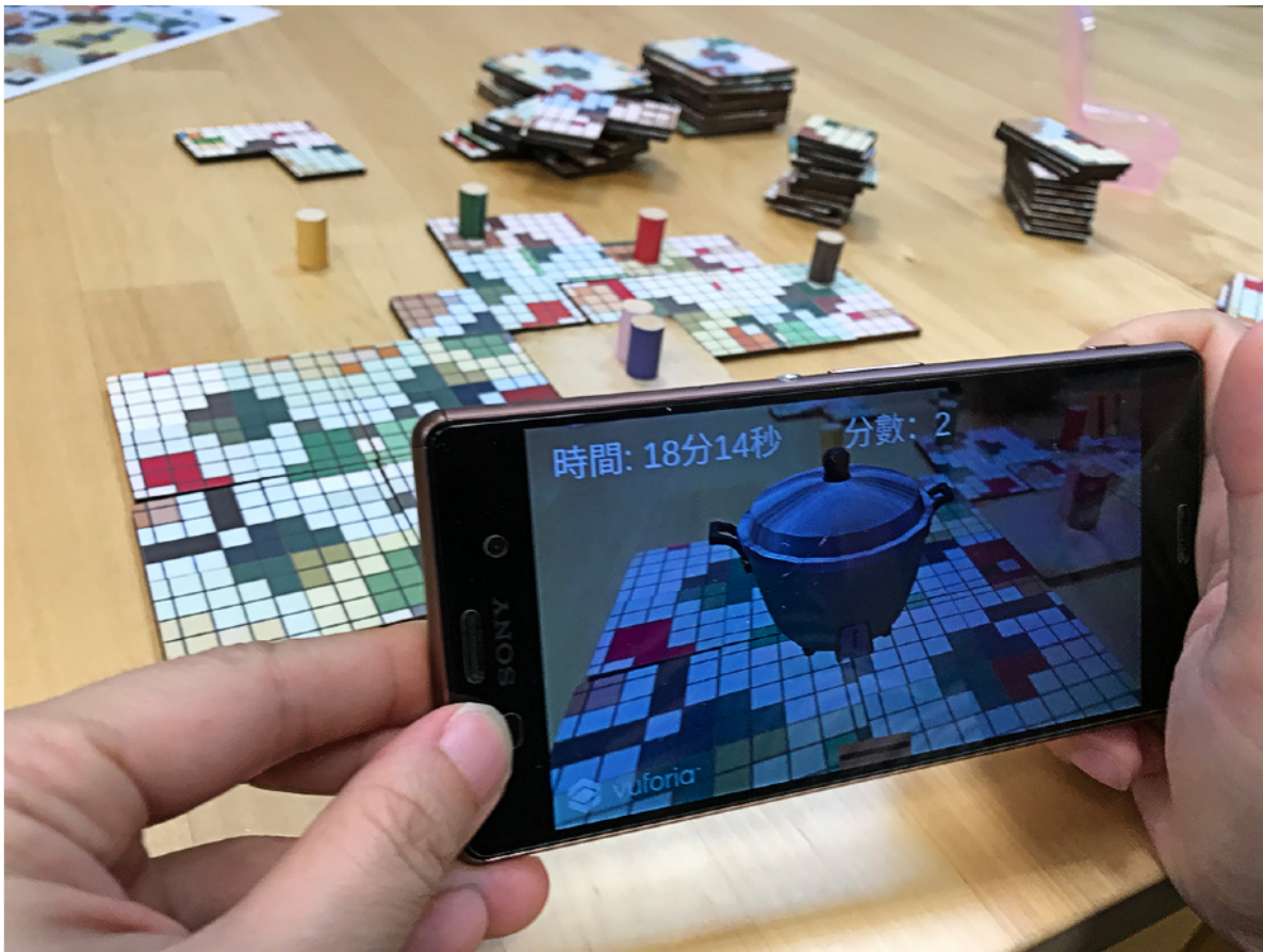
Figure 4. The three-dimensional object of one of the nostalgic artifacts, an automatic cooker and steamer, is presented on the screen of a mobile device when the pattern of the puzzle tiles is assembled correctly.
