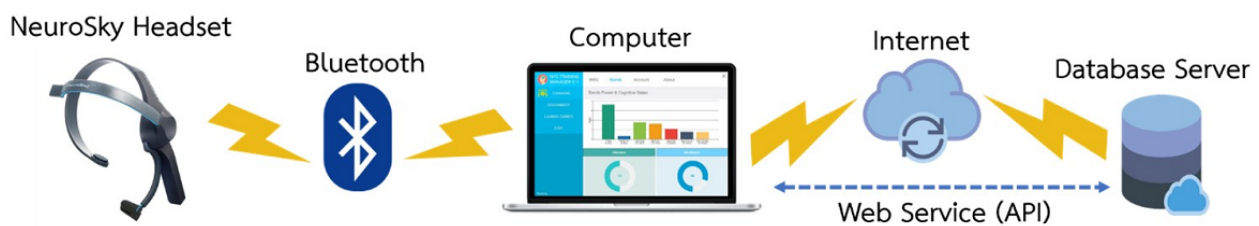
Figure 1. System overview. API: application programming interface.
