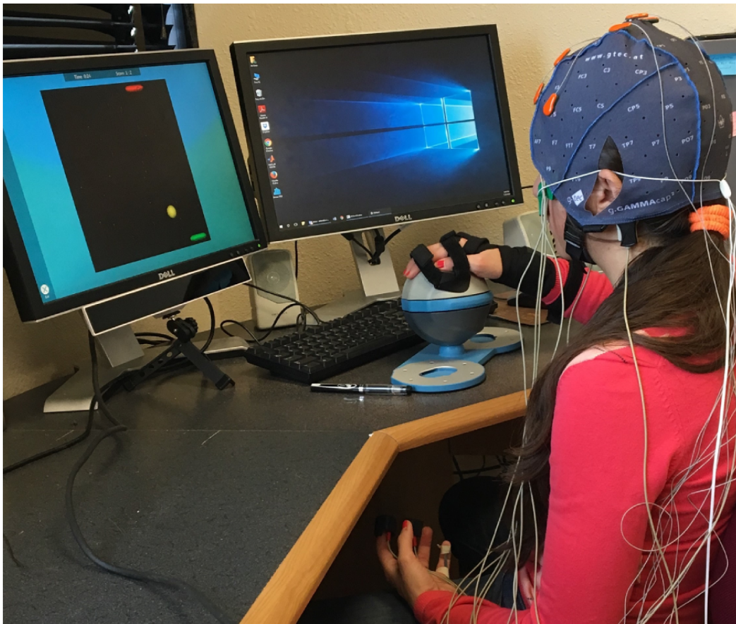
Figure 1. A participant playing the exergame (on the screen) using the Bimeo device (right hand) while wearing the different physiological sensors on the head and nondominant hand. The eye tracker is visible below the screen.
