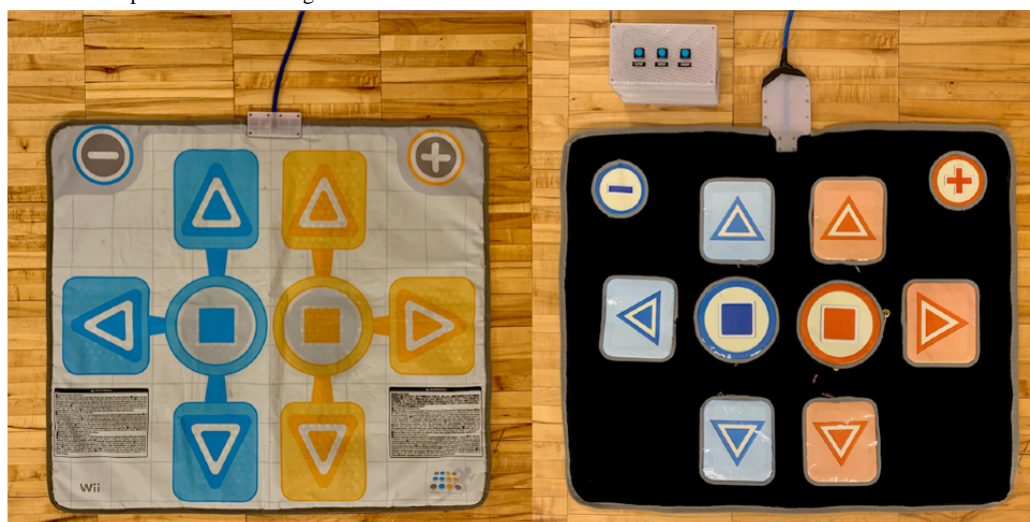
Figure 1. Adapted foot gaming mat (left) and adapted hand (right) mat. Note, the exterior shell of the foot mat looks identical to an off-the-shelf mat, given that only the inside components were re-engineered.
