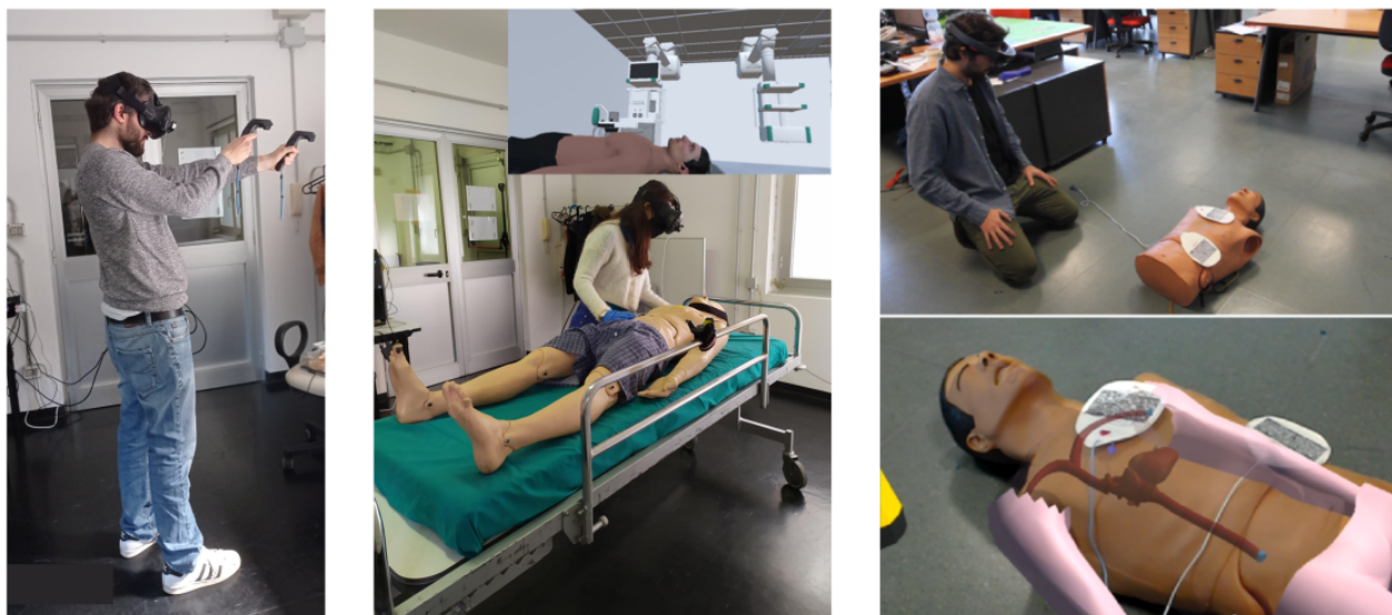
Figure 2. Examples of immersive tools. Left: VR application without haptic feedback. Center: MR system which combines an HMD with a manikin for a more realistic simulation experience. Right: AR application (Holo BLSD) designed to augment a physical manikin with a virtual representation [75]. AR: augmented reality; HMD: head-mounted display; MR: mixed reality; VR: virtual reality.
