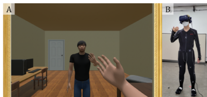
Figure 1. Virtual environment (A) and experimental settings (B) of this study. (A) illustrates the virtual environment from the participant’s perspective. A virtual mirror was set in front of the participant’s location. (B) illustrates the experimental setting of each participant, where each participant wears a motion-capture suit with 37 reflective markers attached and a head-mounted display for observing their virtual avatar’s movement in first-person perspective.
