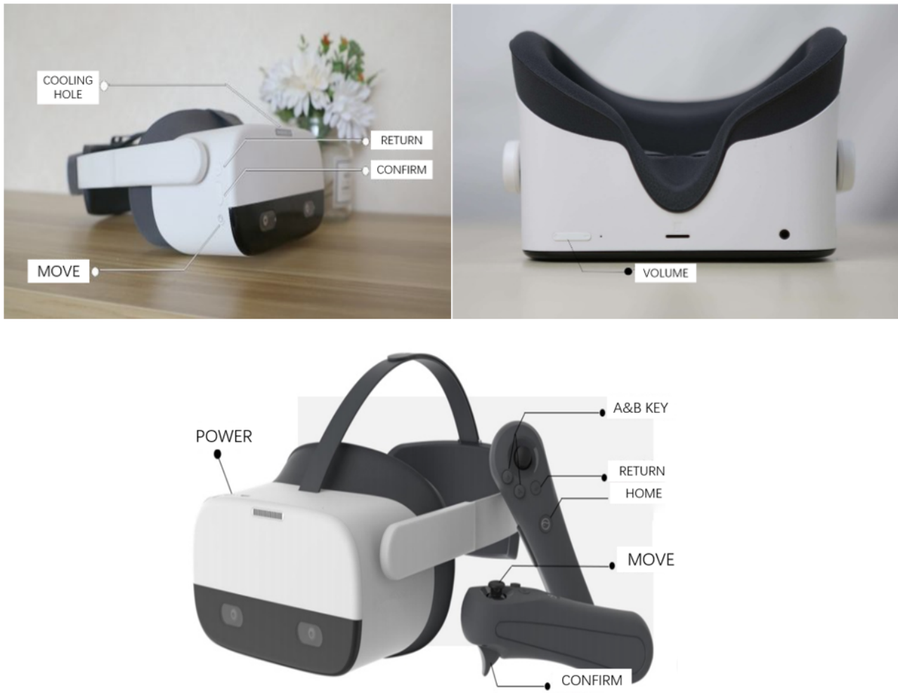
Figure 2. Display of handle, headset, and function key in the device.
