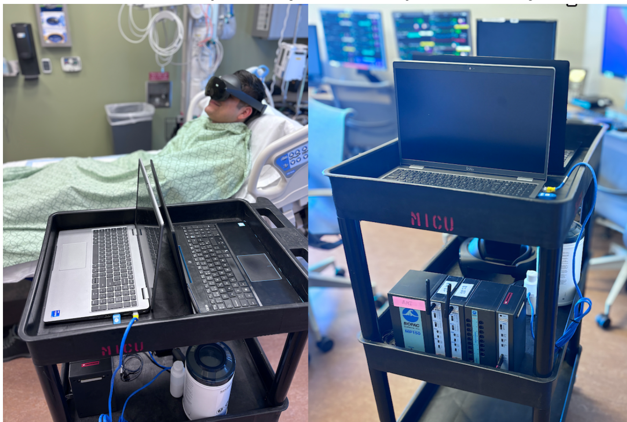
Figure 1. Experimental setup, as demonstrated by study personnel. Two laptops were used to ensure the adequacy of monitoring, project the real-time virtual reality experience of the patient to troubleshoot any technical issues or adverse effects, and to transcribe interview responses after the experience. The Meta Quest headset was chosen out of several possibilities owing to the lack of fabric components to facilitate cleaning after use.
