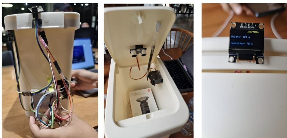
Figure 5. The prototype of the Circonomy smart bin. The prototype connects hardware and software through the node.js/Express REST API server to handle communication between the ESP32 in the smart bin and the Android app. ESP32 serves as a microcontroller to communicate with other modules (such as the load cells, ultrasonic sensors, and servo motors) using the REST API server to send and receive data. API: application programming interface.
